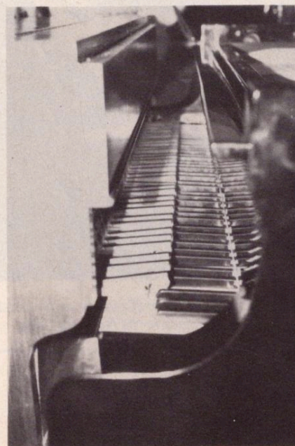
The Ampico reproducing piano fits over the keyboard of a grand piano and plays the keys via fingerlike levers. Two larger levers play the pedals.
