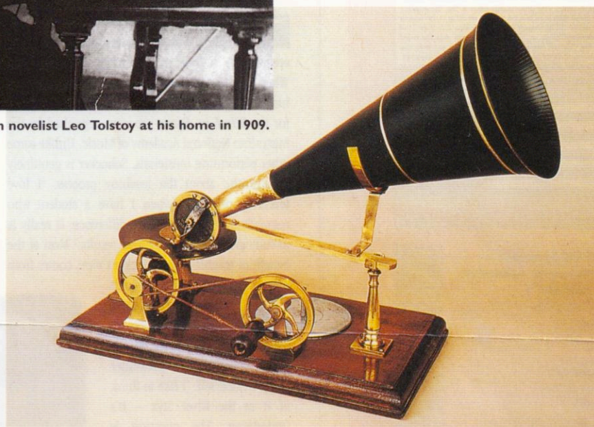
A Berliner 'Gramophone'. An example of the machine as marketed between 1889 & 1893.
